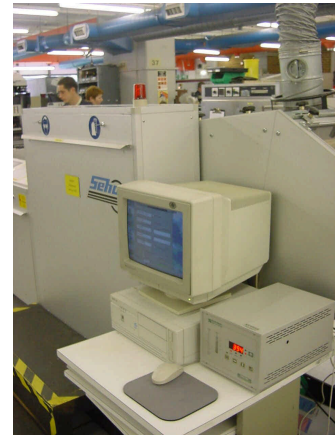
Systech NitroSave oxygen control system in operation at Axis Electronics
